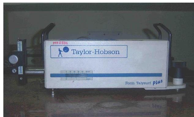
Fig. IV: Profilometer used for measurement of surface roughness (Ra).
